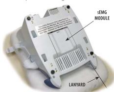
**NOTE:** Do not remove the sEMG. Module, if installed. The sEMG Module will not interfere with installation of the Channel 3/4 Electrotherapy Module
