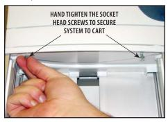
**NOTE:** Secure the System to the cart by tightening the screws by hand only. Do not use a wrench to tighten the screws. Overtightening may cause damage to the System or Module housing.
