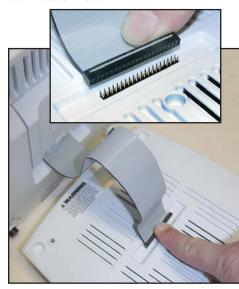
**NOTE:** Ribbon cable must be as shown! Make certain Ribbon Cable is completely seated to Module Connector Pins.
