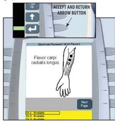
**NOTE:** As illustrated, the two Black electrodes represent Active electrodes and the one White electrode represents the Reference electrode.
