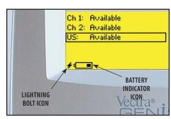
**NOTE:** The Lightening Bolt icon will continue to display as long as the System is connected to a power source.
