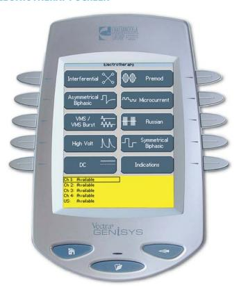
The screen allows the operator to access, set up, and modify parameters of each of the available waveforms within the Vectra Genisys Therapy System. The following pages give a general explanation of a treatment setup.
